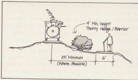
Cross-section of trail path showing use of thorny barriers.
